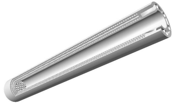
(FIGURE 1: MICROREACTOR BASF/ KIT WITH INTERNAL CHANNELS/ CROSS SECTION)
